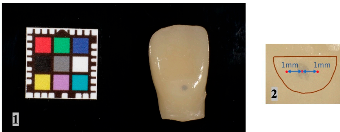
Figure 3. Photographic analysis. 1: Photographed using Casmatch. 2: CIE L^*a^*b^* was recorded at the center of the cavity and 1 mm mesial and distal to the center of the cavity.
