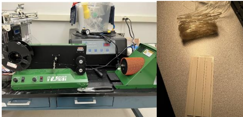
Figure 23 (a) Melt extrusion of PLA/CNF masterbatch, (b) Filament used for 3D printing mechanical test specimens.
