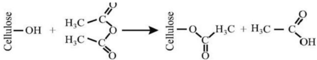
Figure 18. Acetic anhydride reaction with a primary hydroxyl group
