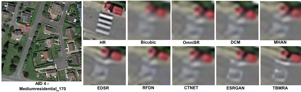
Fig. 4: Comparison of different models on the AID test data for 4 \times SR.
