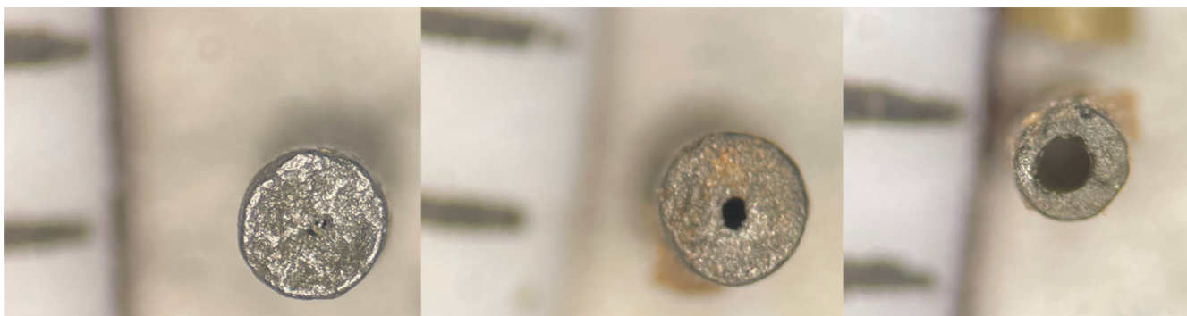
FIGURE 2 Photographs of IMR 4064 particles pre-blast (left), recovered from a PVC device (middle), and recovered from a steel device (right) with 1 mm scale [Color figure can be viewed at wileyonlinelibrary.com ]
