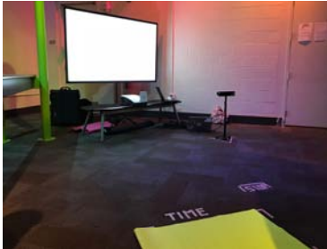
Figure 2: Experimental setup that we used for this study. Our system (IDEA) included a data visualization projected on a 65" screen, a Microsoft Kinect, and some instrumentation of the interaction space (e.g., we use a yoga mat to highlight the area in which users were able to control the timeline).
