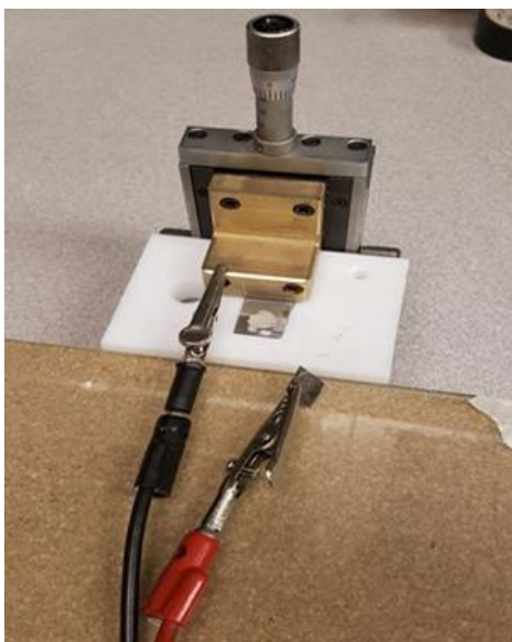
Figure 3.10 A custom-built polling station with adjustable top electrode, developed by Aaron Mosey, used to switch ferroelectric PVDF-HFP polarity. The bottom Au electrode is attached via a gold wire and connected to the power supply.
