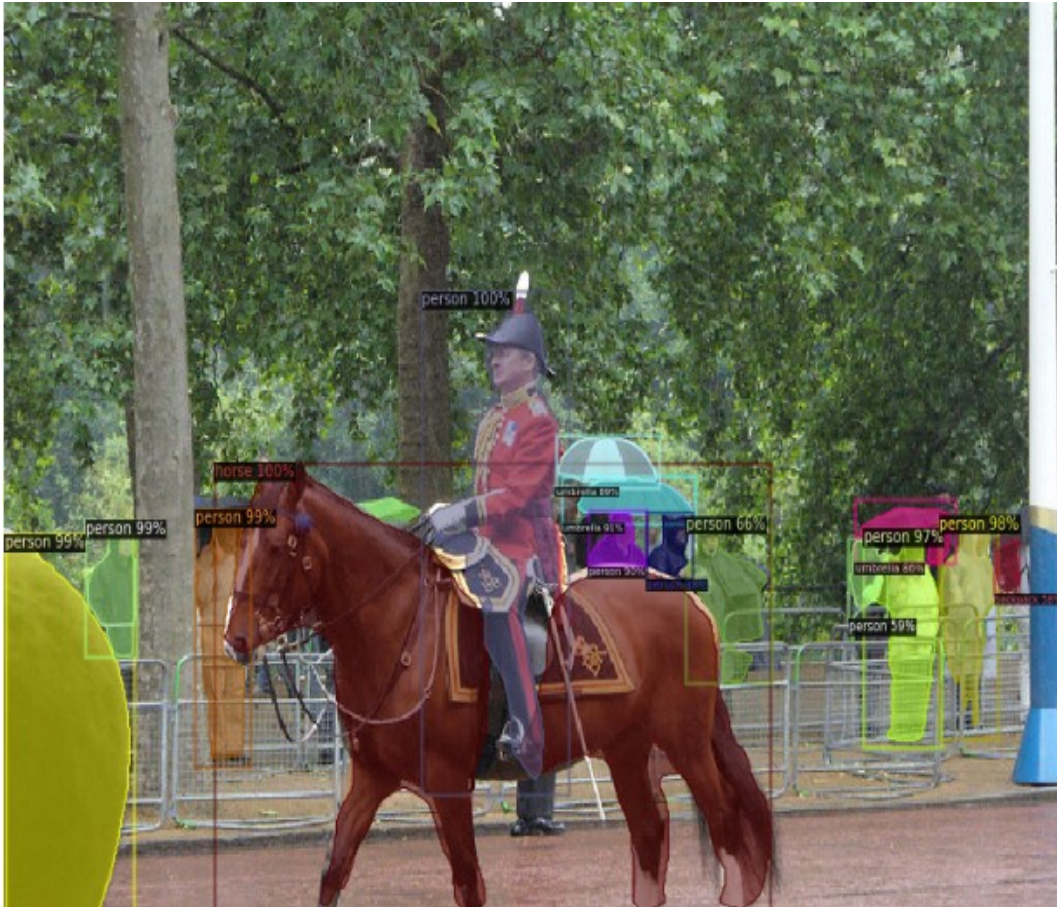
Figure 4.1. Detection of persons from an image using Detectron-2 library [33].
