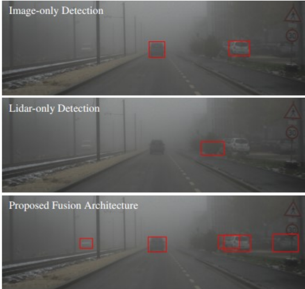
Figure 1.1. Comparison of lidar-only and image only data with their fusion[2].
