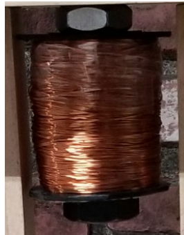
Figure 8: Pictured on the left is the electromagnet mounted in the project enclosure. On the right is the diagram representation of the electromagnet.
