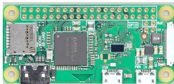
Figure 10: The digital controller will be programmed into a Raspberry Pi Zero W using Python. The Zero W is connected to the A to D converter using the SDA, SCL, +5V, and GND pins. Source: Raspberry Pi, n.d.
