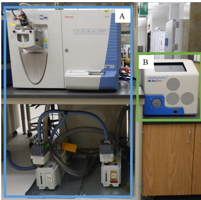
Figure 4.1 Side-by-side of ion trap mass spectrometers, (A) benchtop instrument with two external vacuum pumps, (B) portable instrument with no external equipment.
