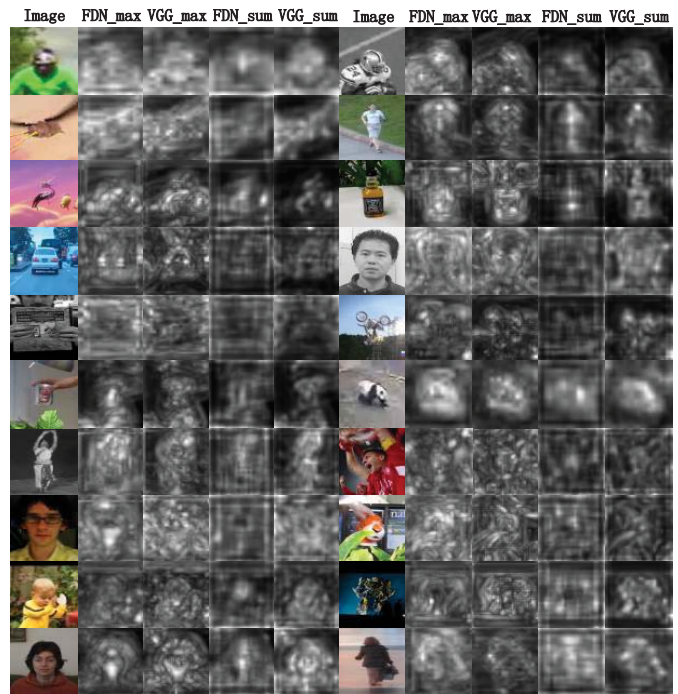
Fig. 4. Visualization of the output conv4-4 features between VGG-19 and FDN. The displaying images come from OTB-100 dataset [88]. The first column is the input image. The second column is taking the max operation among the channel direction of the mimic output features extracted by FDN. The third column is taking the max operation among the channel direction of the intermediate conv4-4 output features extracted by VGG-19. The fourth and the fifth are adapting the sum operation along the channel direction from FDN and VGG-19 network, respectively. The output features are all normalized by dividing the maximum value for visualization.
