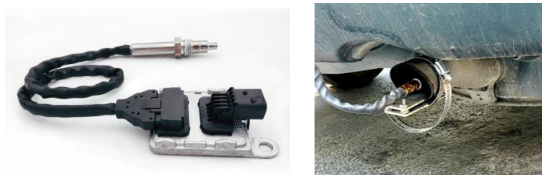
Figure 2: Wi-NOx Sensor Mounted on Tailpipe
