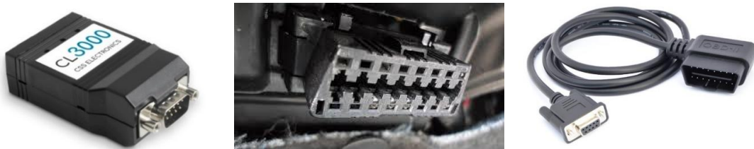
Figure 3: CAN-BUS Logger (CL3000), OBD-II Port and DB9 Adapter Cable
