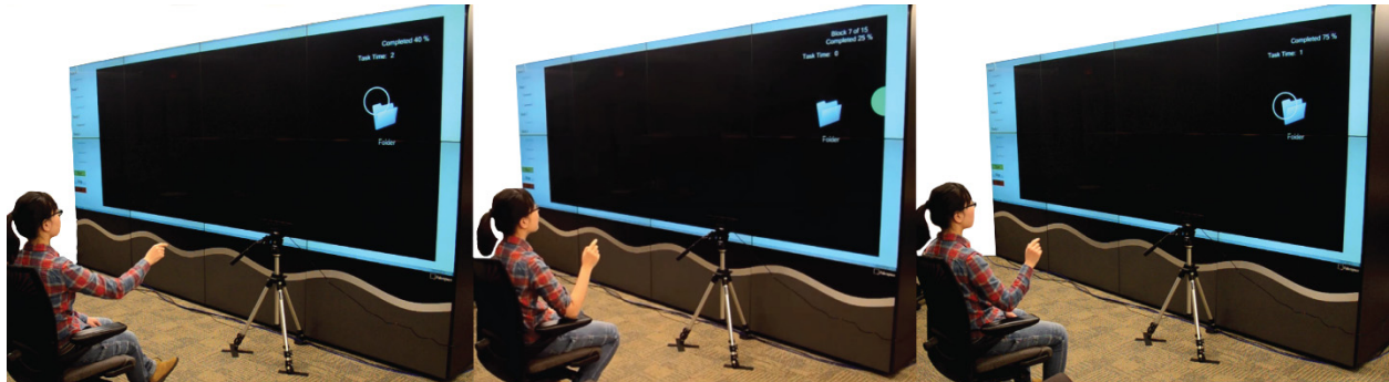
Figure C1. A user points in mid-air to a target folder on a large display (left); Stoppers provide visual feedback as the user's gesture goes out of the display range (center) and guide her back within the display range (right).
