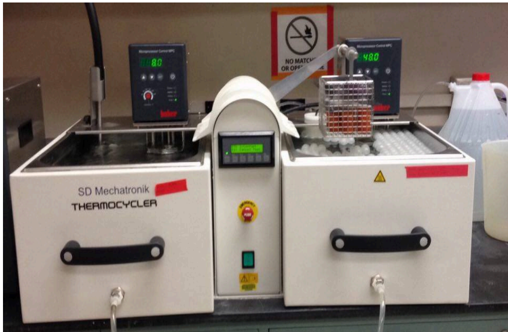
FIGURE 4. Image of thermo-cycling unit.
